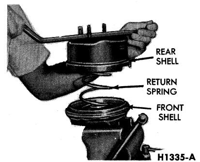
FIG. 17—Separating Booster Shells
